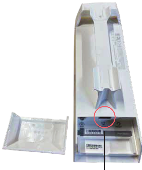
Ethernet connection from PoE
